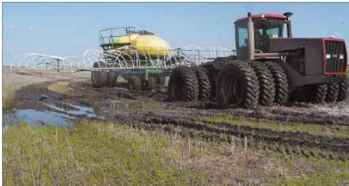
Barry Reimer invented a broadcast spray boom when wet and flooded land stopped him from seeding his fields. | KIM LANGEN PHOTO
